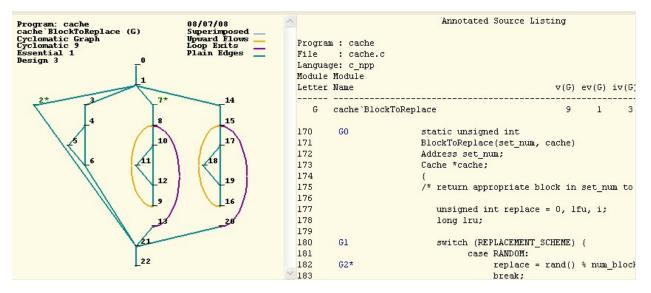
Analysis of the module control flow diagram identifies ways that sources could combine with targets to cause problems. A *Cyclomatic Complexity* measurement of ten (10) means that 10 Minimum Tests will:
